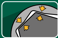
Socket features off-corner loading to reduce fastener rounding
