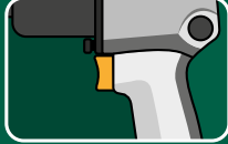
Variable speed trigger
