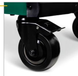
Heavy-duty casters with 5"x 2" PP wheels, 2 fixed and two 360° swivel with top brakes
