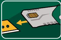
Slide button allows for quick, tool-free blade change
