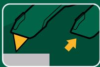
Blade automatically retracts when it loses contact with the material being cut
