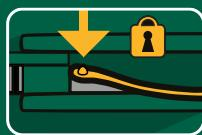
Inner lock mechanism provides secure locking of blade
