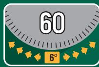
Microdriver needs only a 6° arc to turn fasteners
