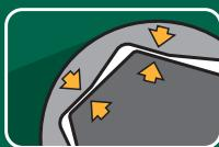
Off-corner loading design reduces fastener rounding
