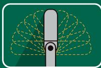
11-position flexible head with locking positions for maximum access
