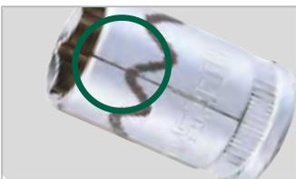
The obvious slippage on socket end or crack on socket wall indicates that this impact tools has been used on this socket. When you are working with impact tools, please choose impact sockets with black coat.
