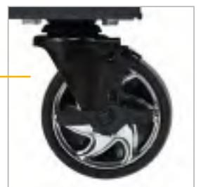
Heavy-duty 5"x 2" steel and PP wheels with pin rolling bears, 2 fixed and 2 360° swivel with top brake
