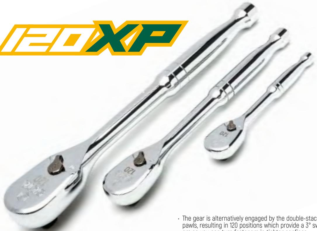
• The gear is alternatively engaged by the double-stacked pawls, resulting in 120 positions which provide a 3° swing arc so you can turn fasteners in tighter confines
