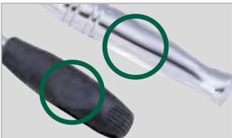
The obvious dent or electroplate desquamation indicates that a pipe wrench or hammer (or other form of "cheater") has been abused on this ratchet. Please use a larger size of ratchet to increase the leverage of any wrench.
