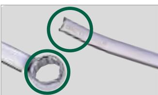
Distort or breach on the wrench is also result of using the wrench as a pry bar. Please use the right pry bar for prying.
