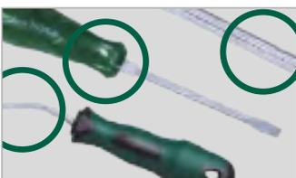
The breach of handle, blade chip-off and bent shanks are the results of using screwdriver as a pry bar, punch or chisel.
